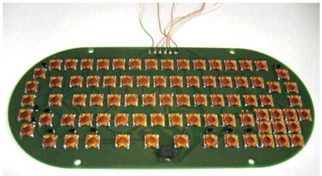
The pushbuttons are small enough to fit right under the key caps - but the total height has to be checked.
