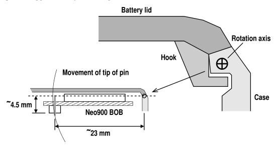
The cover has a hook that goes into an opening in the case. When opening or closing the cover it rotates around that hook, which results in anything mechanically connected to the cover to perform the same rotation.
