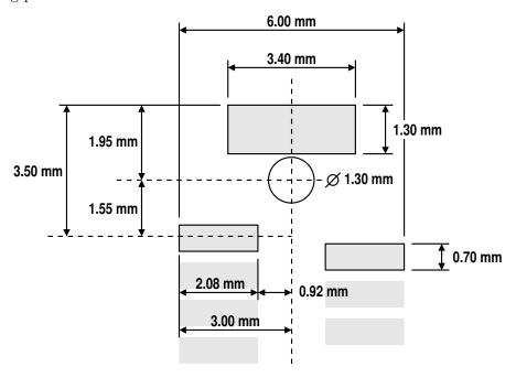
DF9/M40 (above) is generally larger than Conan (below) and places the positioning pins on the center line.
