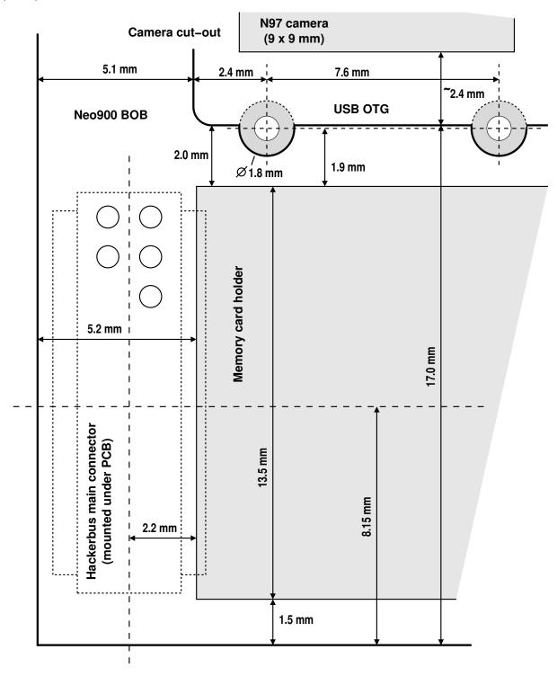
The main connector is soldered to the bottom of the BOB and the header pins pass through holes in the PCB, entering the receptacle from the bottom. The USB OTG contacts are on the LOWER board of Neo900 and can be accessed through an opening in the BOB.
