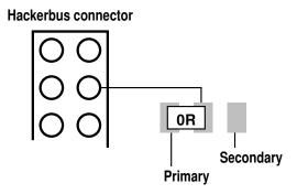
The user can unsolder the resistor and either re-solder it such that it connects to the secondary function, or use jumper wires for any other type of connection.
