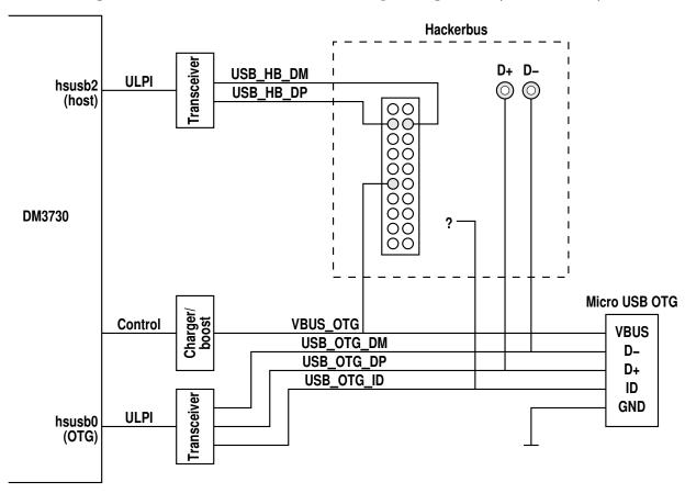
**TO DO:** Define and indicate alternate pin assignment for USB ID.
