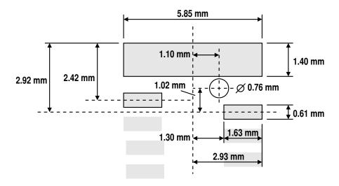
From the above we can derive a common footprint design that should be able to accommodate either type of connector, permitting postponing the component choice until shortly before production and thus reducing sourcing risk:
