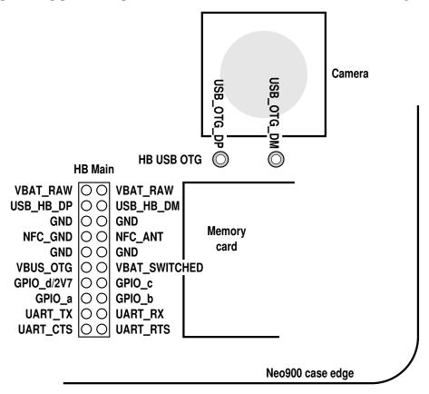
The following table describes the functions of the pins on the Hackerbus main connector:
