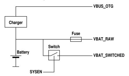
Note that the presence of this fuse does not guarantee that loads exceeding the trip current will not lead to malfunction. Furthermore, the battery is a user-provided item and needs to be evaluated separately by prospective users of VBAT\_RAW. The maximum current available on VBAT\_RAW depends not only on the fuse but also on the characteristics and condition of the battery.
