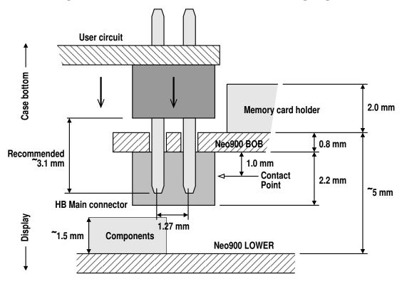
The male header shown as an example in the drawing has the dimensions of the FCI 20021111-00020T4LF through-hole connector,<sup>2</sup> with a contact length of 3.05 mm and a plastic mold height of 2.5 mm. (See also [3].)
