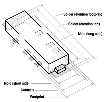
For the long sides we have the length of the body, and the edge-to-edge distance of metal tab and footprint of the solder retention. The body length is either the length of the plastic mold (in the case of Conan, where the mold protrudes) or the distance between the ends of the solder retention tabs (DF9/M40, where the tabs protrude), whichever is larger.
