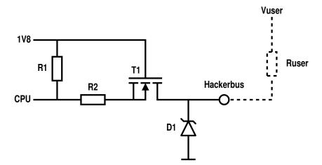
The principle of operation is briefly described in [5] and further details can be found in [6]. R1 is usually an internal pull-up resistor in the CPU of 10 k $\Omega$  or higher. R2 limits the current when CPU and external circuit drive the Hackerbus signal in a conflicting way. R2 is 100  $\Omega$ . D1 protects against ESD and polarity inversion.
