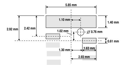
From the above we can derive a common footprint design that should be able to accommodate either type of connector, permitting postponing the component choice until shortly before production and thus reducing sourcing risk:
