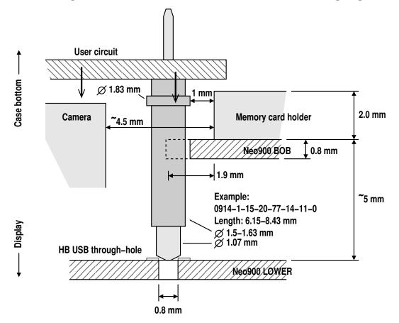
The characteristics of the pogo pins depend on the placement of the user board. Clearances and hole diameters are designed for the Mill-Max 914 series. [4] The following table shows minimum, middle, and maximum length of the pogo pins in this series. The length corresponds to the distance between the facing sides of LOWER and the user board.
