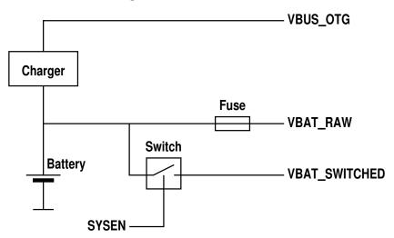
Note that the presence of this fuse does not guarantee that loads exceeding the trip current will not lead to malfunction. Furthermore, the battery is a user-provided item and needs to be evaluated separately by prospective users of VBAT\_RAW. The maximum current available on VBAT\_RAW depends not only on the fuse but also on the characteristics and condition of the battery.
