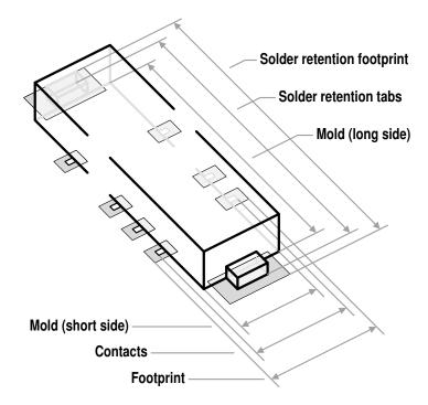
For the long sides we have the length of the body, and the edge-to-edge distance of metal tab and footprint of the solder retention. The body length is either the length of the plastic mold (in the case of Conan, where the mold protrudes) or the distance between the ends of the solder retention tabs (DF9/M40, where the tabs protrude), whichever is larger.
