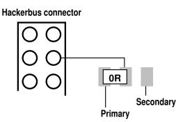
The user can unsolder the resistor and either re-solder it such that it connects to the secondary function, or use jumper wires for any other type of connection.
