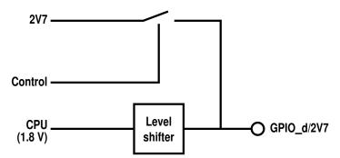
The connection to the CPU is protected by the same circuit as all other IOs available on the Hackerbus. When GPIO\_d is configured as power rail, the CPU should set the corresponding GPIO to High-Z without pull-up or -down. The CPU may read the GPIO, but the resulting value is undefined.
