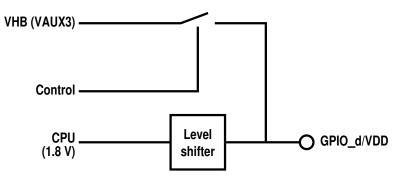
VAUX3 provides up to 200 mA. The voltage can be set by software to 1.5, 1.8, 2.5, 2.8, or 3.0 V.
