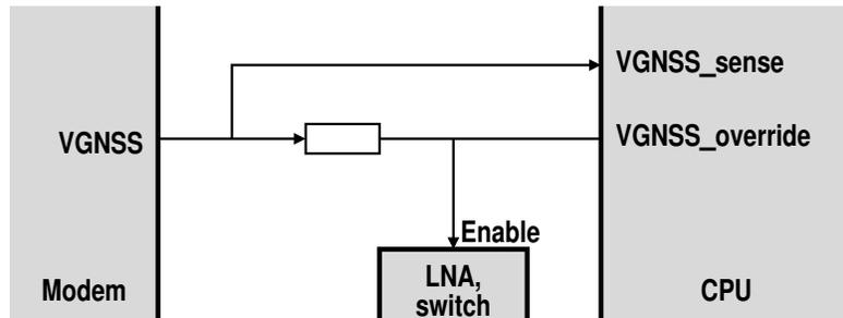
If the CPU tri-states VGNSS\_override, the modem controls the LNA and the GPS kill switch. The CPU “kills” GPS by driving VGNSS\_override low. In either case, VGNSS\_sense tracks which configuration the modem requests.
