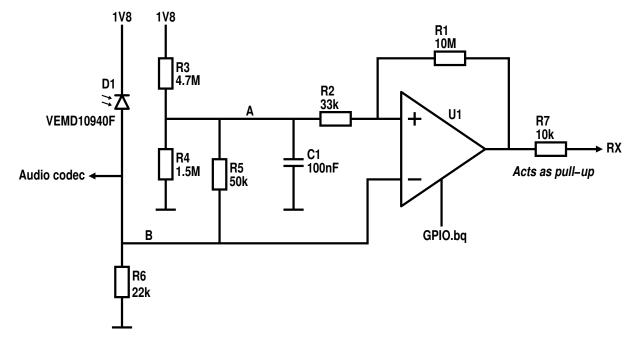
D1 is reverse-biased through R6. R6 pulls the signal at  $\mathbf{B}$  close to ground when the diode is not illuminated, and lets the voltage raise when D1 is illuminated and the reverse current through it increases.
