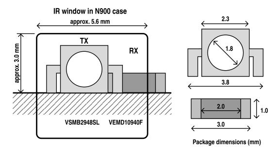
The transmitter should be closer to the window since its performance is more important than that of the receiver.
