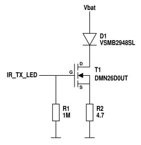
The maximum continuous forward current of the IR LED (VSMB2948SL) is 100 mA. We design the circuit to operate at no more than 90 mA, so that even a LED accidently left turned on permanently will not overheat.
