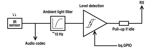
The series resistor ensures that CPU and Hackerbus can override the IR receiver. When the receiver is not illuminated or when it is disabled, the circuit outputs a high level and thus acts as a pull-up for the RX line.
