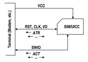
The terminal (modem, etc.) first applies the lowest available voltage to the SIM card. The card may then send an ATR message on the serial interface using CLK and I/O. If the terminal receives no message, it switches to the next higher voltage, waits again for an ATR message, and so on.
