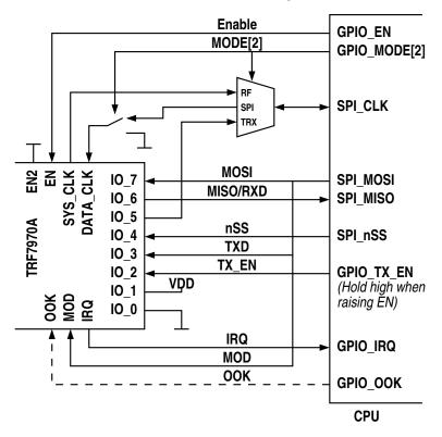
Note that IO\_5 is an active if useless output also in SPI mode and therefore must be separated from SPI clock generated by the host. The following table shows the different clock configurations:
