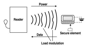
If the application requires a SE, then this may be provided either as part of the smartphone's hardware, by software, or through a Subscriber Identity Module (SIM) card. In the latter case, the NFC/RFID subsystem acts merely as a relay between the radio interface and the SIM card, with the SE controlling most of the protocol processing. We discuss the mechanism used for communication between the secure element in the SIM card and the smartphone in section 6.
