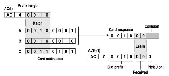
From a card's point of view, the sequence ends when the prefix matches the entire address of the card (in which case the AC command is called SELECT) and the card then acknowledges this with a SAK (select acknowledge) response.
