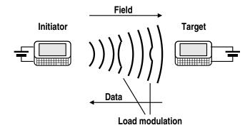
The above is called "passive" mode. Since both devices are capable of producing an electromagnetic field, there is also an "active" mode, depicted below.
