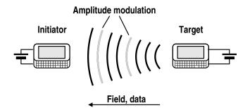
In this mode, the initiator deactivates its field when it is done sending and the target generates its own field to send a response. I.e., this is how radio communication normally works, with each party providing the electromagnetic field needed for its transmissions.
