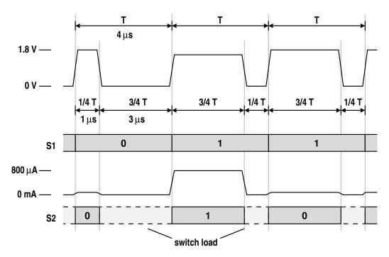
The card switches its load characteristics while SWIO is low, and the state of S2 is only defined while SWIO is high. Further details can be found in section 8 of [23].
