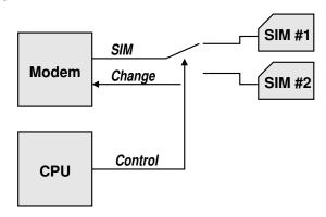
In addition to the card change signals from the SIM cards, the hardware generates a card change indication before the switch is operated.
