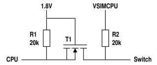
For simplicity, we can also use the same type of level shifter for RST and CLK, given that they use the same voltage levels and operate at the same or a lower frequency.
