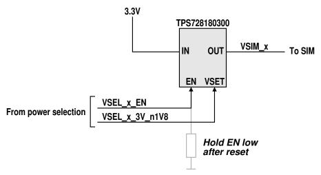
This regulator outputs either 1.8 V or 3.0 V. When disabled, it discharges its output through a  $60~\Omega$  resistor.
