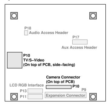
Except for the S-Video connector P4 and the camera connector P10, all are on the bottom of BB-xM. P4 is a side-facing mini-DIN connector from which we can feed the analog TV output signal to Neo900 v2.
