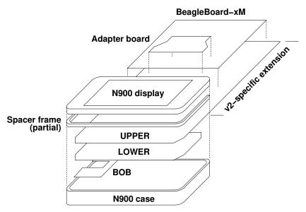
There are three principal boards of v2 proper: the LOWER board contains most of the peripherals, including modem, WLAN/BT, and audio. LOWER interfaces mechanically with the N900 case. The UPPER board has the keyboard, the display connector, the camera interfaces, and some sensors. Memory card, the flash LEDs, and a few sensors are on BOB (the Break-Out Board). BOB also features the Hackerbus interface [2] that connects to user-provided external circuits.
