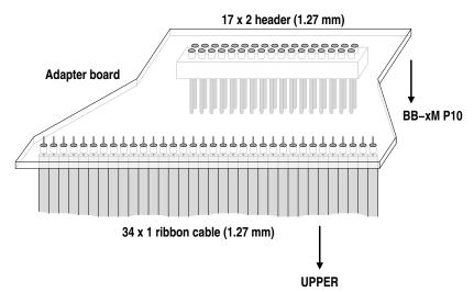
The exact size and shape of the board is to be determined by layout. Note that some signals on the P10 are not used by v2 or are redundant, so the ribbon cable could have less than 34 conductors.
