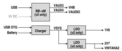
A 5 V DC adapter (regulated) can be used instead of USB to provide BB-xM with power. While we do not expect to need this, we show it as a possible choice.
