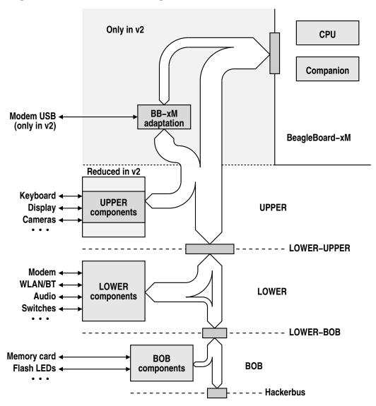
Since BB-xM does not provide all the functionality we need, UPPER of v2 also contains circuits for adapting and extending what BB-xM provides. These adaptations are discussed in more detail in section 4.
