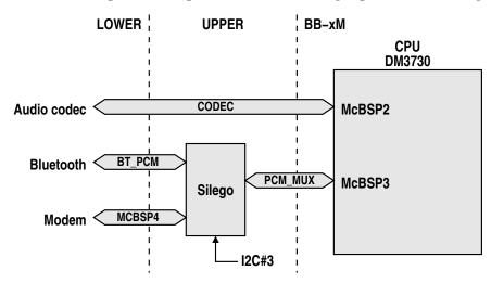
The Silego chip is configured through I<sup>2</sup>C.
