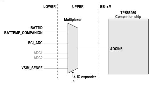
The analog multiplexer is configured through three control signals from the v2-specific IO expander (see section 4.4).
