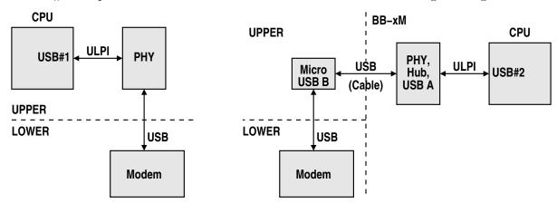
Since there is no CPU and therefore no ULPI bus on v2, we instead add a Micro USB B connector that can be connected to any regular USB port – e.g., one of the USB ports of BB-xM, as shown on the right-hand side of the above drawing.
