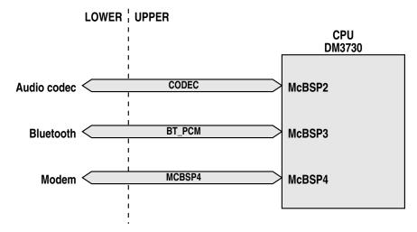
BB-xM only gives access to two of these ports. We therefore share McBSP3 between Bluetooth and modem, and insert a Silego mixed-signal matrix to act as programmable multiplexer:
