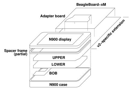
There are three principal boards of v2 proper: the LOWER board contains most of the peripherals, including modem, WLAN/BT, and audio. LOWER interfaces mechanically with the N900 case. The UPPER board has the keyboard, the display connector, the camera interfaces, and some sensors. Memory card, the flash LEDs, and a few sensors are on BOB (the Break-Out Board). BOB also features the Hackerbus interface [2] that connects to user-provided external circuits.
