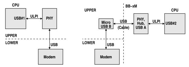
Since there is no CPU and therefore no ULPI bus on v2, we instead add a Micro USB B connector that can be connected to any regular USB port – e.g., one of the USB ports of BB-xM, as shown on the right-hand side of the above drawing.
