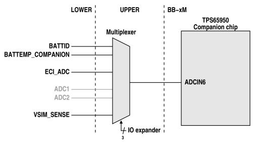
The analog multiplexer is configured through three control signals from the v2-specific IO expander (see section 4.4).
