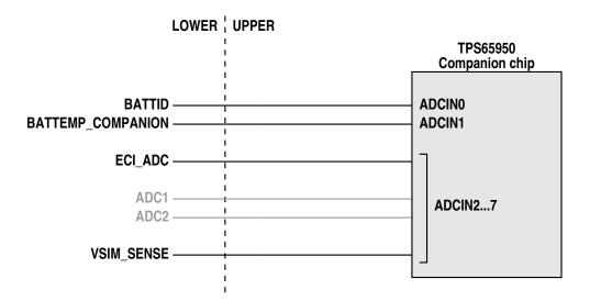
BB-xM only provides a single ADC input, ADCIN6 on the Auxiliary Expansion Header. While this limits the use of at least some of the signals, we can still monitor them for correct levels. To that end, v2 uses an analog multiplexer to select which of the available analog signals gets sent to the BB-xM:
