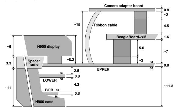
Dimensions are in mm. The drawing is only approximate and some artistic liberties have been taken especially in the horizontal direction. Further details on the stacking of items in Neo900 can be found in [4].
