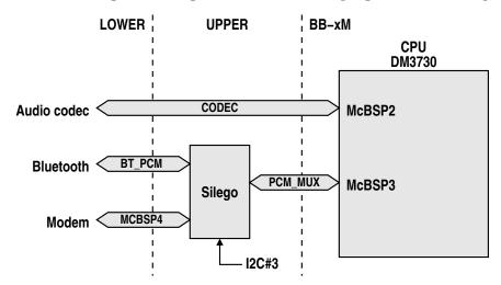
The Silego chip is configured through  $I^2C$ .
