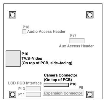
Except for the S-Video connector P4 and the camera connector P10, all are on the bottom of BB-xM. P4 is a side-facing mini-DIN connector from which we can feed the analog TV output signal to Neo900 v2.
