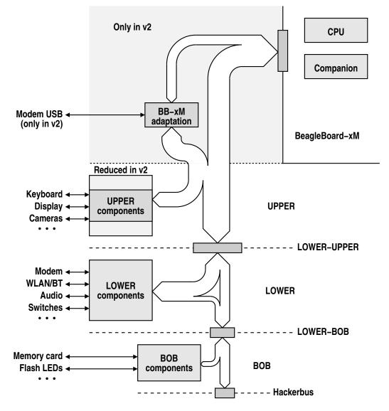
Since BB-xM does not provide all the functionality we need, UPPER of v2 also contains circuits for adapting and extending what BB-xM provides. These adaptations are discussed in more detail in section 4.
