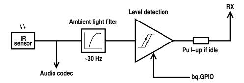
The series resistor ensures that CPU and Hackerbus can override the IR receiver. When the receiver is not illuminated or when it is disabled, the circuit outputs a high level and thus acts as a pull-up for the RX line.
