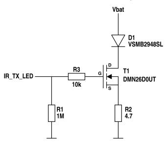
The maximum continuous forward current of the IR LED (VSMB2948SL) is 100 mA. We design the circuit to operate at no more than 90 mA, so that even a LED accidently left turned on permanently will not overheat.
