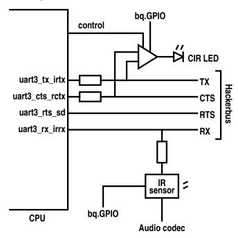
The signal named bq.GPIO is not only a control input but it also determines the configuration after CPU reset. It is described in section 3.1.
