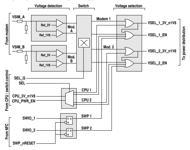
Since power can be requested by various entities, we do not route modem power directly through the switch but instead measure the voltage the modem outputs and request the corresponding voltage from the following stages. (Block "Voltage detection".)
