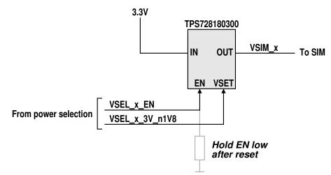
This regulator outputs either 1.8 V or 3.0 V. When disabled, it discharges its output through a 60  $\Omega$  resistor.
