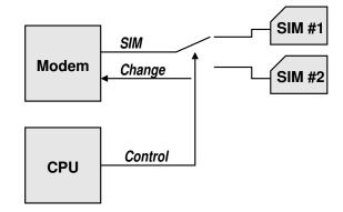
In addition to the card change signals from the SIM cards, the hardware generates a card change indication before the switch is operated.
