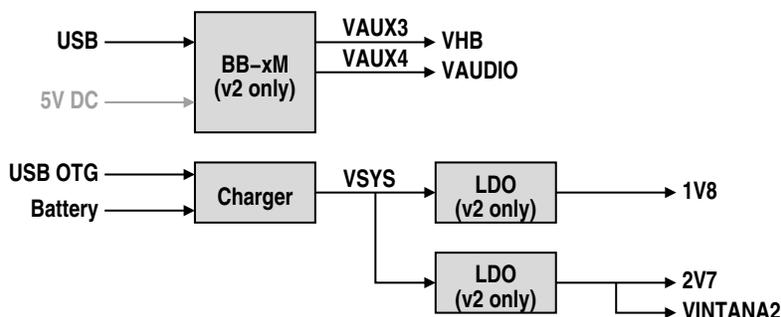
A 5 V DC adapter (regulated) can be used instead of USB to provide BB-xM with power. While we do not expect to need this, we show it as a possible choice.
