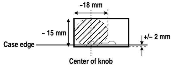
The exact location and width of the finger holes should be determined from the placement of the respective switches on the PCB, which is outside the scope of this document.
