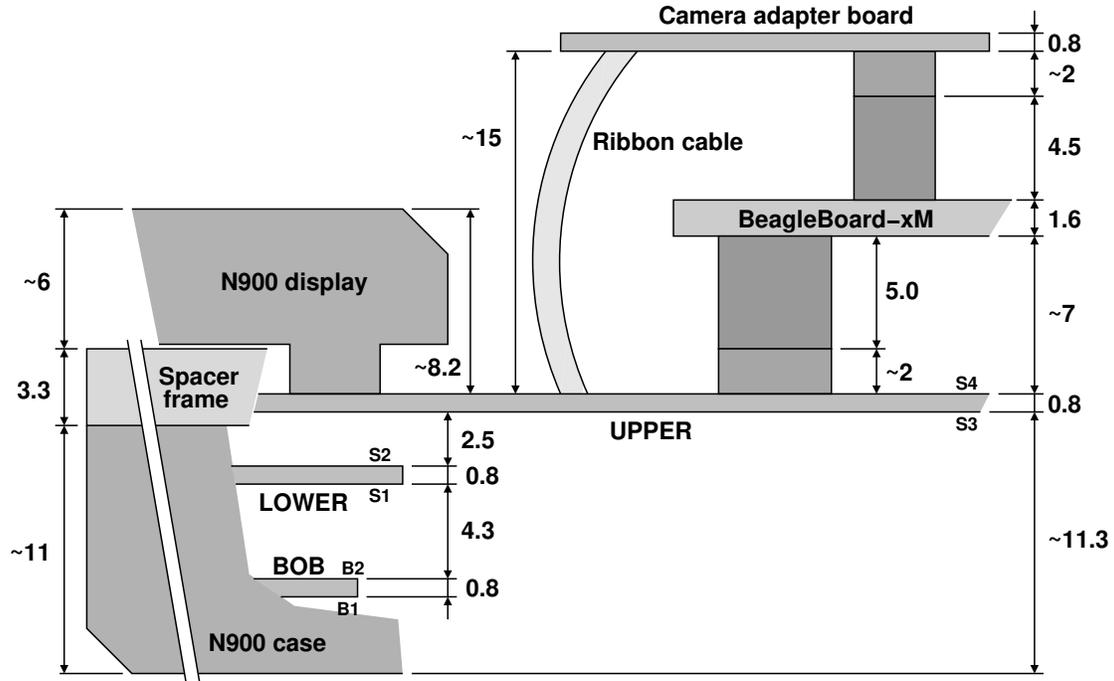
Dimensions are in mm. The drawing is only approximate and some artistic liberties have been taken especially in the horizontal direction. Further details on the stacking of items in Neo900 can be found in [4].
