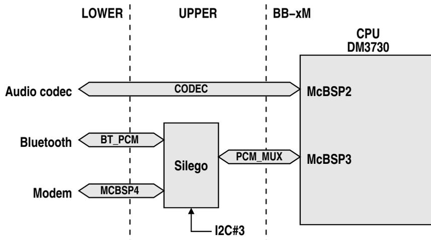
The Silego chip is configured through I<sup>2</sup>C.
