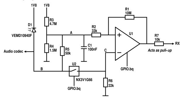
When the receiver is enabled (analog switch U2 is closed), D1 is reverse-biased through R6. R6 pulls the signal at **B** close to ground when the diode is not illuminated, and lets the voltage raise when D1 is illuminated and the reverse current through it increases.
