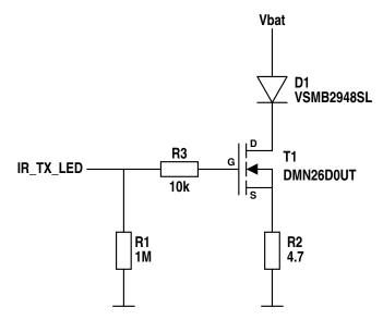
The maximum continuous forward current of the IR LED (VSMB2948SL) is 100 mA. We design the circuit to operate at no more than 90 mA, so that even a LED accidently left turned on permanently will not overheat.
