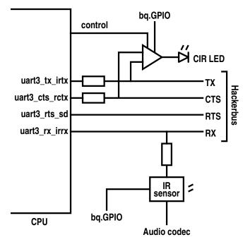
The signal named bq.GPIO is not only a control input but it also determines the configuration after CPU reset. It is described in section 3.1.
