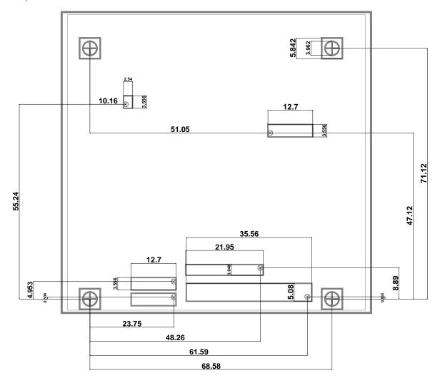
The board is shown from above. The position of the board edges relative to the mounting holes is only an approximation.
