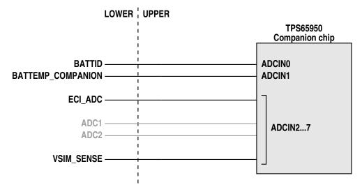
BB-xM only provides a single ADC input, ADCIN6 on the Auxiliary Expansion Header. While this limits the use of at least some of signals, we can still monitor them for correct levels. To that end, v2 uses an analog multiplexer to select which of the available analog signals get sent to the BB-xM:
