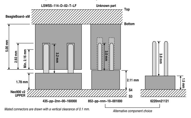
We select the following parts to mate with the BB-xM connectors:
