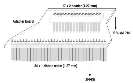
The exact size and shape of the board is to be determined by layout. Note that some signals on the P10 are not used by v2 or are redundant, so the ribbon cable could have less than 34 conductors.
