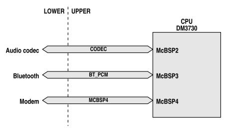
BB-xM only gives access to two of these ports. We therefore share McBSP3 between Bluetooth and modem, and insert a Silego mixed-signal matrix to act as programmable multiplexer:
