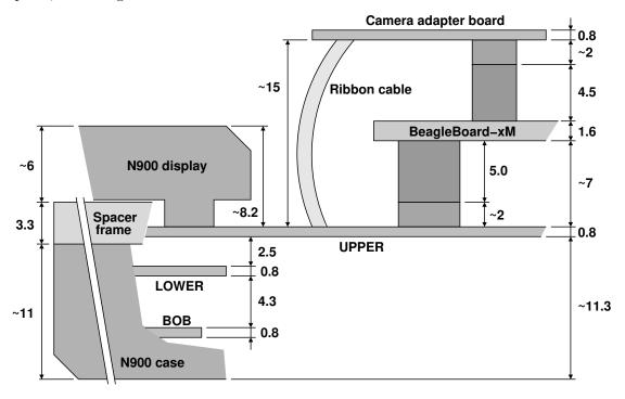
Dimensions are in mm. The drawing is only approximate and some artistic liberties have been taken especially in the horizontal direction. Further details on the stacking of items in Neo990 can be found in [4].
