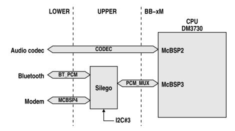
The Silego chip is configured through  $I^2C$ .
