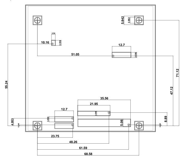
The position of the board edges relative to the mounting holes is only an approximation.
