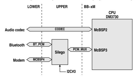
The Silego chip is configured through I<sup>2</sup>C.
