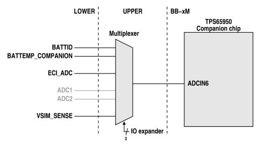
The analog multiplexer is configured through three control signals from the v2-specific IO expander (see section 4.3).
