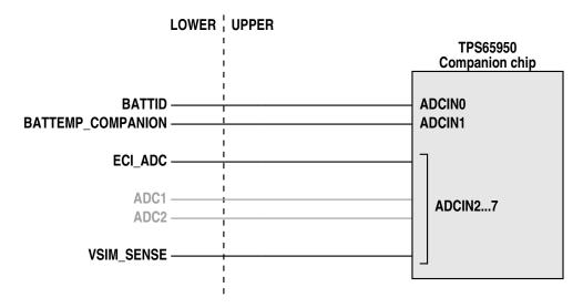
BB-xM only provides a single ADC input, ADCIN6 on the Auxiliary Expansion Header. While this limits the use of at least some of signals, we can still monitor them for correct levels. To that end, v2 uses an analog multiplexer to select which of the available analog signals get sent to the BB-xM:
