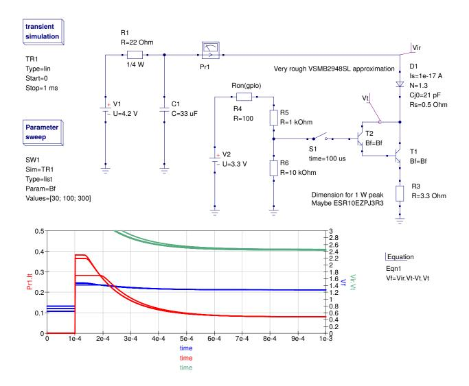
Example current-limiting circuit: continuous current through the IR LED D1 is limited by R1 and R3. Short pulses in the 100  $\mu$ s range can draw extra current from C1. The peak current is then limited by the constant current transistor circuit. This example uses a Darlington configuration to obtain a current gain  $\beta \gg 100$ .
