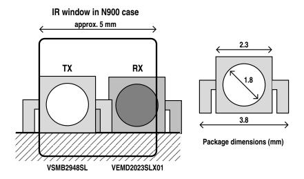
The transmitter should be closer to the window since its performance is more important than that of the receiver.
