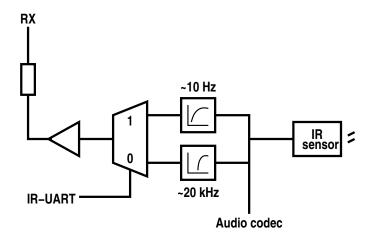
Given that IR-UART can have very long high or low pulses, a high-pass filter with a much lower cut-off frequency has to be used when IR-UART mode is selected. A cut-off frequency of about 1–100 Hz should be sufficient for DC blocking. The figure above illustrates the concept.
