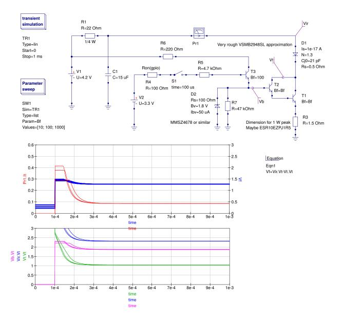
Example current-limiting circuit: continuous current through the IR LED D1 is limited by R1 and R3. Short pulses in the 100  $\mu$ s range can draw extra current from C1. The peak current is then limited by the constant current transistor circuit. This example uses a Darlington configuration to obtain a current gain  $\beta \gg 100$ .
