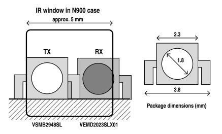
The transmitter should be closer to the window since its performance is more important than that of the receiver.
