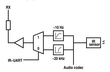
Given that IR-UART can have very long high or low pulses, a high-pass filter with a much lower cut-off frequency has to be used when IR-UART mode is selected. A cut-off frequency of about 1–100 Hz should be sufficient for DC blocking. The figure above illustrates the concept.
