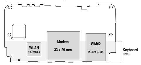
The basic idea is to place these components under the keyboard area. When typing on the keyboard, the PCB flexes a little. This causes mechanical stress on chips and solder joints that may eventually lead to device failure. We therefore want to avoid placing components under the keyboard on S3, especially no large chips.
