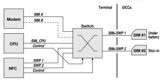
We use A/B for the buses that are affected by the switch, and 1/2 for the SIM side and for signals or buses that are not affected by the switch.
