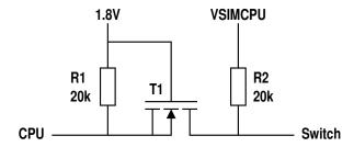
For simplicity, we can also use the same type of level shifter for RST and CLK, given that they use the same voltage levels and operate at the same or a lower frequency. In order to reduce the circuit footprint and the number of components, integrated level shifters from the TI LSF family [6] could be used instead of the discrete circuit shown above. The programmable pull-up resistors built into the CPU can be used for R1, further reducing the component count.
