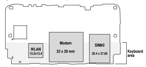
The basic idea is to place these components under the keyboard area. When typing on the keyboard, the PCB flexes a little. This causes mechanical stress on chips mounted on the other side of the PCB, and on their solder joints. Such stress may eventually lead to device failure. We therefore want to avoid placing components under the keyboard on S3, especially no large chips.
