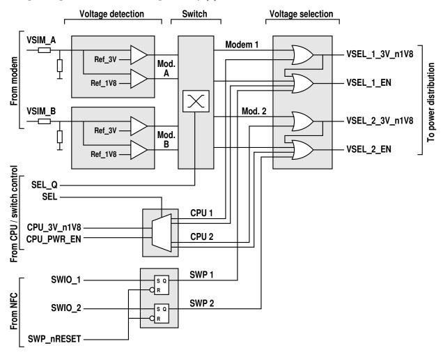
Since power can be requested by various entities, we do not route modem power directly through the switch but instead measure the voltage the modem outputs and request the corresponding voltage from the following stages. (Block "Voltage detection".) Since the analog input voltage must not be greater than VDD, the voltages output by the modem must be divided by at least  $\div 2$ .
